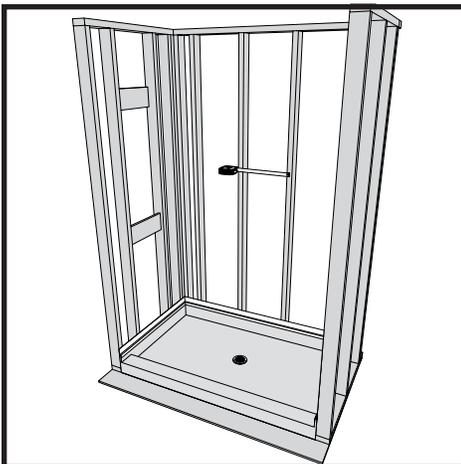
2. Measure the distance between vertical studs. (Please note that the distance between the center lines of 2 adjacent studs generally is 16 inches and the niche is designed for that condition.)
