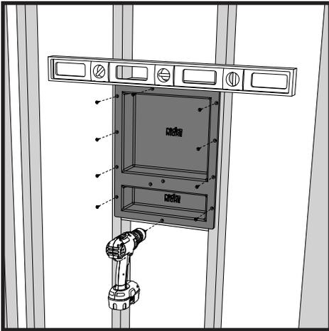
4. Level and mechanically fasten the Redi Niche using one framing screw in each pre-drilled.
