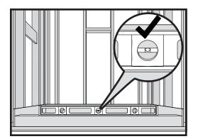
9. Using the level, ensure that the pan is level left to right, and front to back along the splash walls. Also make sure the pan is level left to right along the curb.
