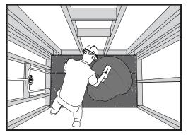
5. Spread your mortar base (should be a milk shake consistency), evenly across the subfloor at the thickness calculated in Step 4.
