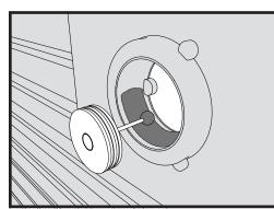
7. If there is access from the subfloor below and you followed Step 3a, then brush PVC adhesive on the inside of the drain and outside of the cut drain pipe and quickly insert into drain connection, then be sure the drain pipe extends far enough below the subfloor so it can be connected to the waste water pipe following the installation.
