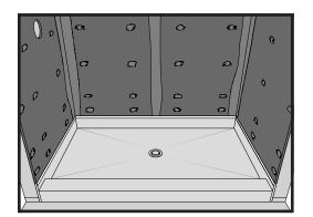
10. Install the shower backer board and water proofing in accordance with the standards established by the Tile Council of North America, Inc. Seal and waterproof joint between backer board and the shower pan splash walls using Redi Flash® or 100% silicone. It is recommended to use a membrane and fluid applied waterproof in addition to the Redi Flash® or 100% silicone. Allow the mortar bed to dry in accordance with the instructions of mortar manufacturer.
