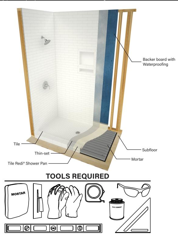
sufficient to fit properly into the shower pan drain connection. 4. Turn the shower pan over and note that there are ribs under the shower pan floor. To calculate the amount of mortar needed, you will need to know the depth of the deepest point in between the ribs. Once you have that value, calculate the thickness (depth) of your mortar base (Type N or S Mortar) using the following formula:
