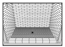
11. Adjust the height of the drain as necessary to accommodate the flooring covering. Set your tile using a white modified thin-set and a notched trowel as specified by your thin-set manufacturer based on your tile size. Tile Redi recommends the modified thin-set products found in table below.
